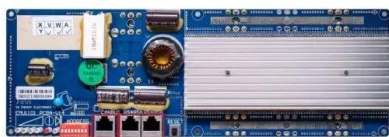
ES485 Communication between battery and inverter Baud rate:9600bps ES485 Interface Communication between parallel packs or EMS and PC Baud rate:9600bps
