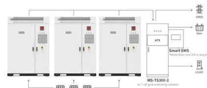
Application scenarios of energy storage battery products
